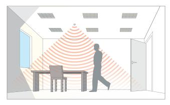
Presence detected, sufficient daylight, lights off.
