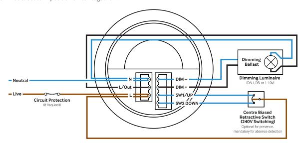
When there is a requirement to have an 'Off' state that results in a low-lit level, then use the DSI / DALI lines as dimming control with an unswitched live feed direct to the ballast. Set the 'Off value' (in the Advanced Programming section) to a value greater than zero to achieve this low-lit dimmed level for the 'Off' state. See the diagram below for wiring details.
