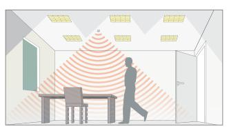
Presence detected, insufficient daylight, all lights on.
