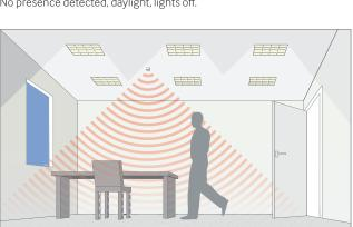
Presence detected, some daylight. Lights on and dimmed to maintain a minimum level.
