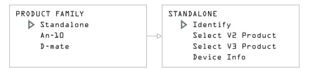
After placing the cursor on Identify, point to the target sensor product and press enter to get to the appropriate menu for programming.
