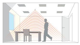
Presence detected, sufficient daylight, lights off.
