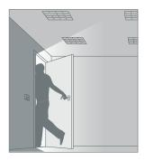
**Absence Detection:** Upon entering the room the person switches on the light as normal, but on leaving the detector switches off the lighting automatically. Lights can also be switched off manually.
