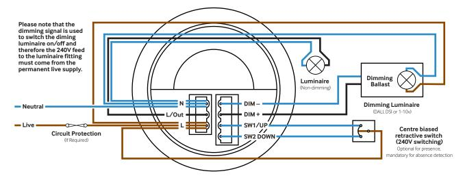
Please note that the centre biased retractive switch will provide control for the dimming luminaire(s) only.
