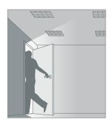
**Presence Detection:** Detectors will switch on lighting automatically when a person enters the room, and switches off lighting automatically when no movement is detected.
