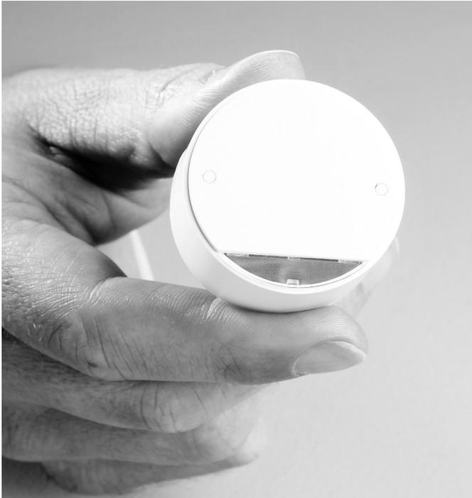
The MWS5 series of miniature microwave presence detectors provide automatic control of lighting loads with optional manual control. As microwave radiation penetrates plastic and glass, this unit has been specifically designed to be mounted inside a luminaire.
