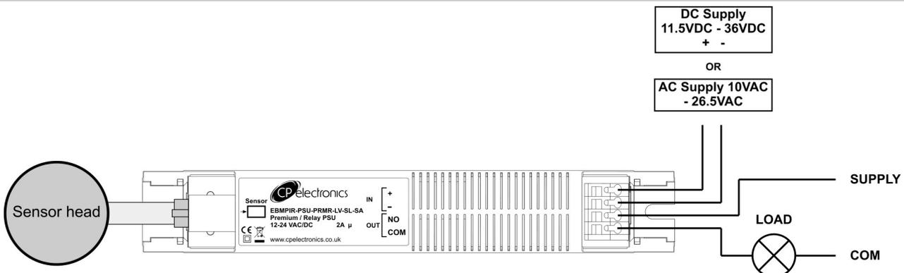
Note. Due to the proximity to other terminals, the low voltage supply (AC or DC) cannot be SELV if the output connections are mains (ie, non SELV).
