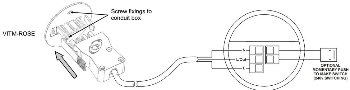
Where absence detection or override is required, wire the switch directly to the detector or use the VITM4 series of marshalling boxes
