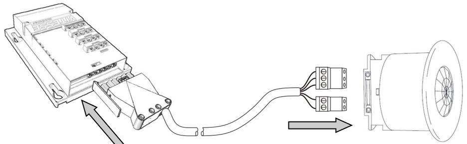
Detector lead supplied with detector.
