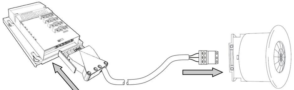
Detector lead supplied with detector.
