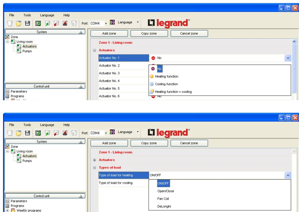
By clicking on each **Pump** (e.g.: Pump No. 1), it is possible to select the type of function required (heating, cooling, heating + cooling or no function) and the activation **Delays**.
