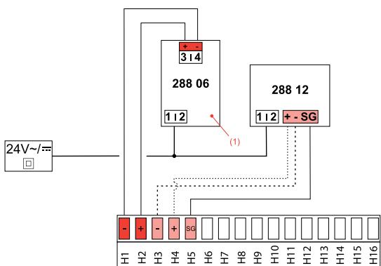
(1) For the correct operation of the 288 12 in this configuration, is mandatory the use of the power supply module 288 06
