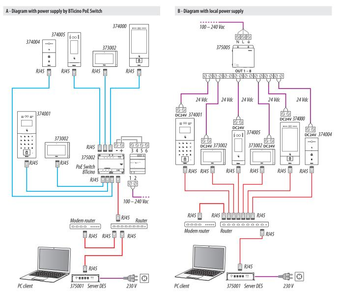
Attention: This device does not support standard POE power supplies, but only POE power supplies identified with 375002. Connect the cat5/5e/6 FTP or cat5/5e/6 UTP cable with ferrite supplied to the connector.
