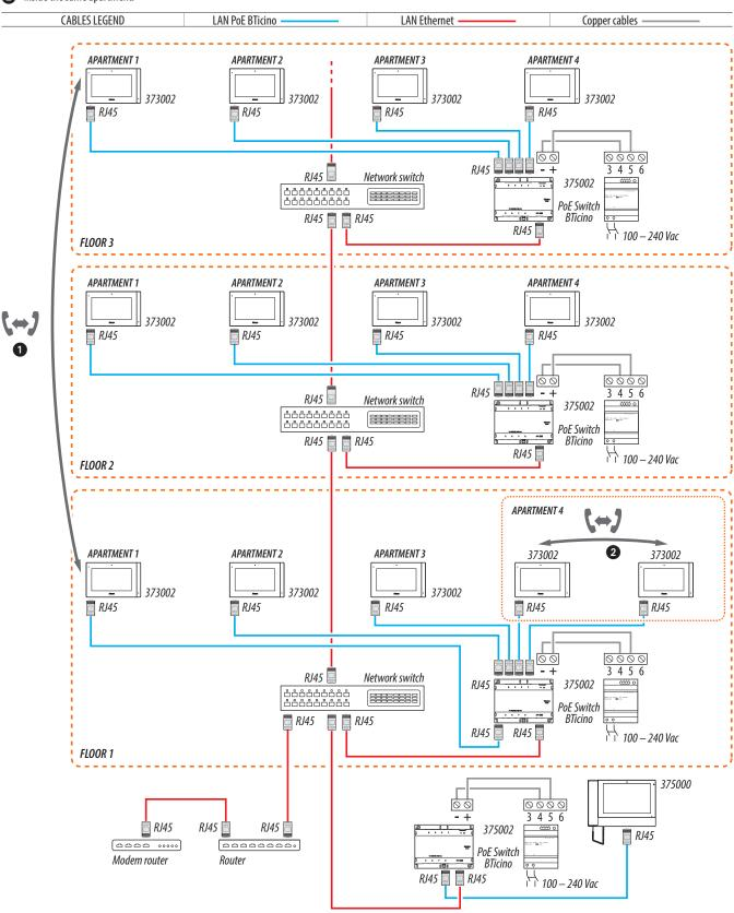
Attention: do not directly connect PoE ports to an unsuitable network interface, such as a device powered by a different voltage. Connect the UP LINK port to a suitable port, never to a PoE port. Note: to connect the devices it is possible to use both types of wiring (diagram A or diagram B) or even mixed ones.
