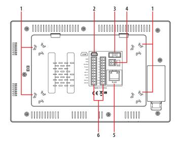
All contacts must be connected to GND and the corresponding dedicated input.
