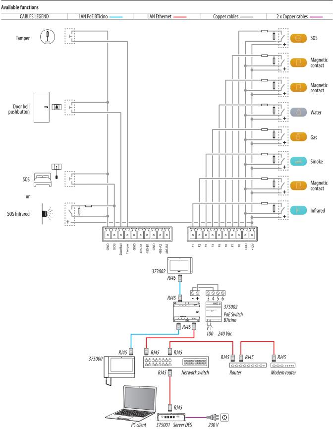
**Attention:** do not directly connect PoE ports to an unsuitable network interface, such as a device powered by a different voltage. Connect the UP LINK port to a suitable port, never to a PoE port. **Note:** the alarm functions are the default ones. It is possible to modify them in the appropriate section.
