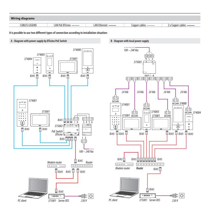
Attention: this device does not support standard POE power supplies, but only POE power supplies identified with 375005. Connect the cat5/5e/6 FTP or cat5/5e/6 UTP cable with ferrite supplied to the connector.
