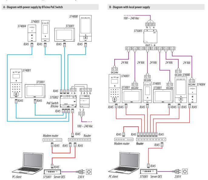
**Attention:** do not directly connect PoE ports to an unsuitable network interface, such as a device powered by a different voltage. Connect the UP LINK port to a suitable port, never to a PoE port. **Note:** to connect the devices it is possible to use both types of wiring (diagram A or diagram B) or even mixed ones.
