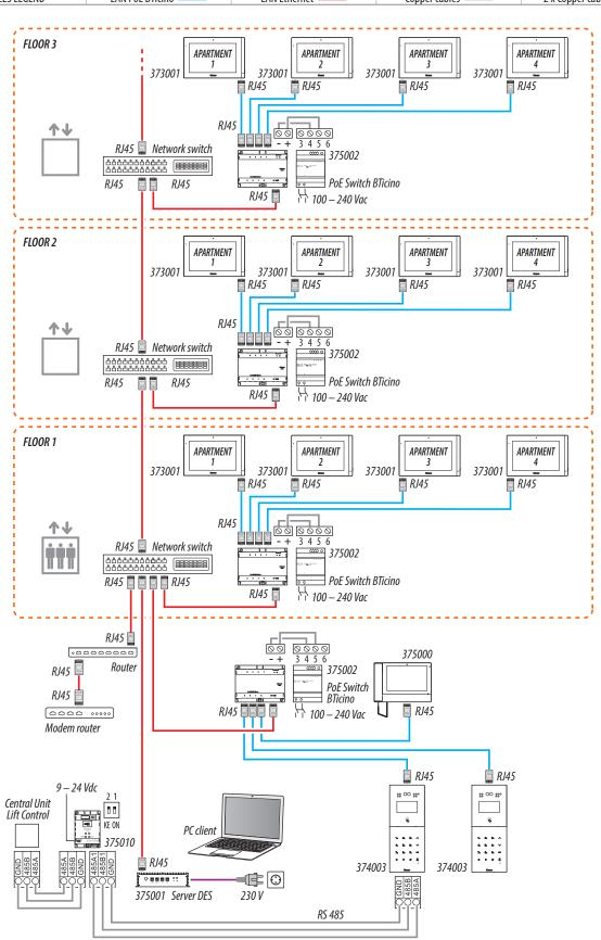
Attention: do not directly connect PoE ports to an unsuitable network interface, such as a device powered by a different voltage. Connect the UP LINK port to a suitable port, never to a PoE port. Note: to connect the devices it is possible to use both types of wiring (diagram A or diagram B) or even mixed ones.
