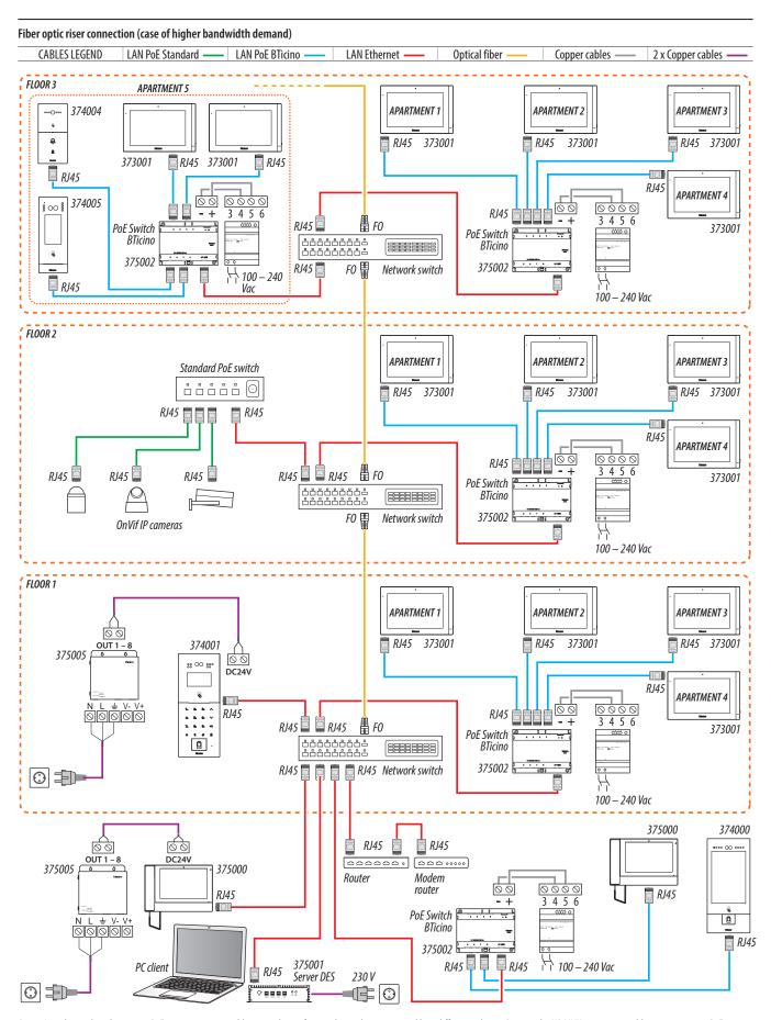
Attention: do not directly connect PoE ports to an unsuitable network interface, such as a device powered by a different voltage. Connect the UP LINK port to a suitable port, never to a PoE port. Note: to connect the devices it is possible to use both types of wiring (diagram A or diagram B) or even mixed ones.
