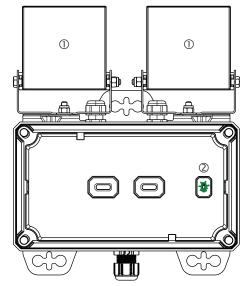
The spotlights are off 0The green unit status LED comes on (flashing while the batteries are charging: 28 hours max.) 0
