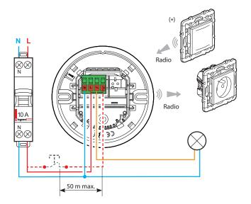
(\*) This product can be controlled by: • A wireless batteryless switch (ON/OFF) Or
