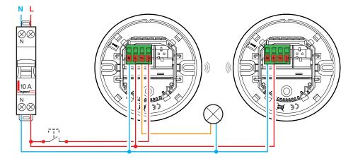
The master can be paired with a maximum of 5 sensors configured as slaves. The slave can extend the detection zone. No loads should be paired with it. If being used in "**Master/Slave**" mode, the wired push-button should only be connected to the "Master" sensor.
