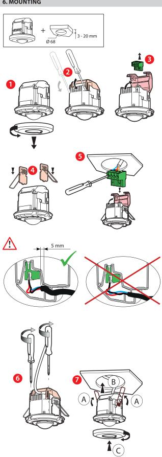
Mounting and wiring must be done with the power off. Please follow the Safety Instructions exactly.
