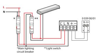
Note: Although self-contained emergency lighting units do not consumemuch power, you must check that the line dedicated to these lighting units can deliver the necessary current. You will find below the current the line needs to withstand for 100 installed lighting units according to the catalogue number (for simplicity, we have assumed just one type of lighting unit is installed per line):
