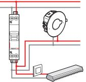
The branch can be joined in the electric cabinet, on the switch or in a junction box. The rules concerning the power supply are the same for emergency lighting as for any other type of luminaire.
