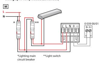
**Note:** Although self-contained emergency lighting units do not consume much power, you must check that the line dedicated to these lighting units can deliver the necessary current. You will find below the current the line needs to withstand for 100 installed lighting units according to the catalogue number (for simplicity, we have assumed just one type of lighting unit is installed per line):
