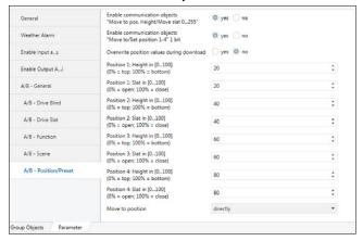
This function allows you set a height position or slat position, directly using with communication object.
