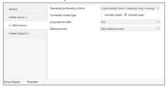
The dual surface shutter function triggers shutter actuators, which can adjustment shutter and blind. You can rise the shutter/adjust the lamella using a single key and lower the shutter/adjust the lamella using a second key surface blind operation. Every shutter actuator controls with a 0-signal the up movement and a 1-signal down movement.
