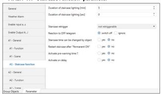
If you want to use staircase function, you must have been enabled 'Staircase' on the function windows. Than required parameters and communication, objects are visible. The staircase function can be parameterized for each channel.
