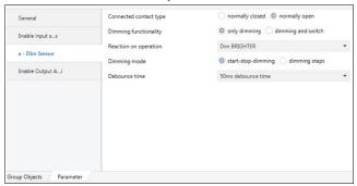
You can use the corresponding input to switch the light on or off or dim it. When dimming, dimming up or dimming down is carried out via the 4 bit dimming object; the parameters for the dimming steps can be set. In addition, you can also transmit the corresponding dimming step cyclically for a period of time that can be set as required.
