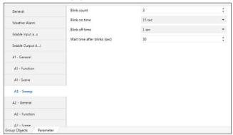
Sweep function only starts to operate if the relay is switched ON. It's an alternative way for turning off the relay with pre-warning. The sweep function is desired to warn a person that lights will go out shortly.
