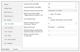
The blind actuator calculates the current position of a blind from the running time. This calculation has to be performed because the drive cannot provide any feedback on its position.
