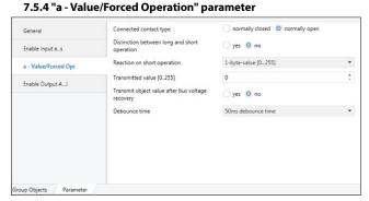
You can use these value/forced functions to parameterize different object actions. You can transmit one or two objects short or long press status sequence, and select the size of the objects required (1 bit, 2-bit priority control, 1 byte, 2 byte or 4 byte) as needed. This enables you to parameterize a large number of application options. You can enter two values and set whether and how they are to be transmitted short or long.
