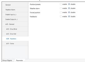
All outputs can be parameterized independent of one other. These parameters are only visible in blind operation.
