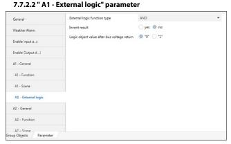
Logic function can be used independently for each output. With this function, the 'Switch' object can be logically linked with the "External logic input". Channel relay switch a result of the logic operation. For example, "Switch" object value 1 and "External logic input" object value 0 relay switch as a result of 1 & 0 operation.
