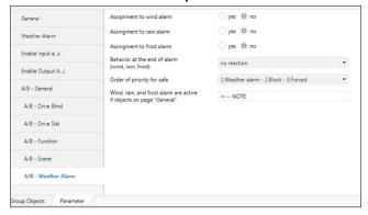
The weather functions must first be globally enabled before they can be parameterized and used. After general weather function is enabled, the weather alarm can be enabled or disabled independently of one other. The reaction at beginning of an alarm telegram is received "1". Alarm function is terminated as soon as a new alarm telegram is received "0".
