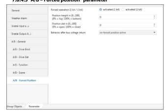
The forced position function can be used for each output. The forced position function has a 1 bit or 2 bit optional communication object. The blind can be moved up or down via forced operation telegram (1 bit or 2 bit). Forced position function can be used for blind cleaning time. It can protect the person for unexpected accident.
