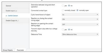
This function is used, for binary inputs to which a switch or a push button is attached, to send a switching telegram (ON, OFF or TOGGLE) as a reaction to a rising and / or falling signal edge at this input. It has only 1 bit communication objects.
