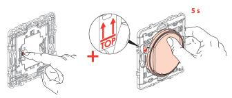
While holding the «setup» button on the wireless, batteryless control, press the upper button for 5 seconds.
