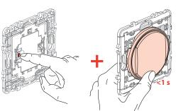
While holding the «setup» button on the wireless, batteryless control, **briefly** press the «Sleep» or «Wake Up» button on the wireless batteryless control.
