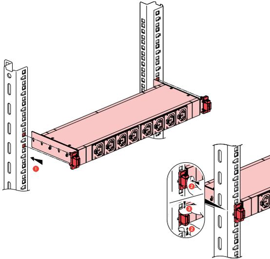
Horizontal mounting with snap-on fixing (for square holes 9.5 x 9.5)
