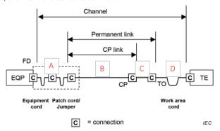
The CP must be minimum 15m from the patch panel: CP link (B)
