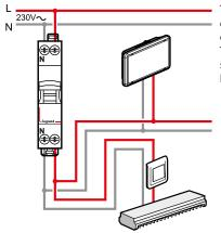
The branch can be joined in the electrical cabinet, on the switch or in a junction box.
