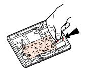
When the batteries have been changed, replace the maintenance label, marking on it the date on which the unit was returned to service.
