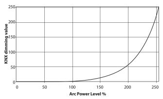
Fig. 16 KNX - DALI - Dimming curve
