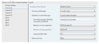
Fig.15 Parameter window "Shutter control, X"
