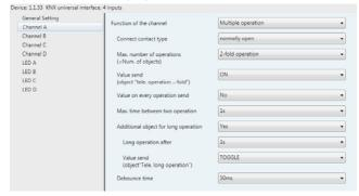
Fig.14 Parameter window "Multiple operation"
