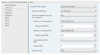
Fig. 6 Parameter window "Value/force output, X" (distinguish with a short and long operation)
