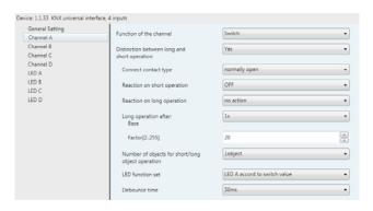
Fig. 4 Parameter window "Switch X" (distinguish between a short and long operation)
