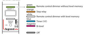
2 - The function is selected by a short press on the push-button. The push-button LED colour determines the chosen function.
