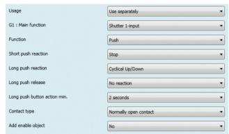
This function allows using just one push button for moving shutter up and down, stopping of the motion and opening and closing of the slats. To achieve this a distinction is made between short and long push action.
