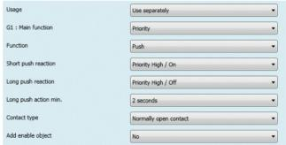
This function is used for inputs with a push button to send a priority telegram, the push is short or long, a telegram is sent.
