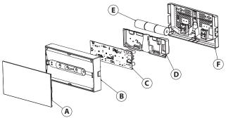
A Diffuser: opal polycarbonate, self-extinguishing 750° 30 s
