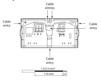
TELEC - Connection terminals: no particular direction of connection with Legrand remote control Cat. Nos. 0 039 00/01. Terminal capacity:  $2 \times 2.5 \text{ mm}^2$
