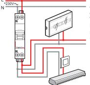
The branch can be joined in the electrical cabinet, on the switch or in a junction box.
