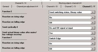
This function is used, for example, to query and transmit the switching status of a signalling contact or the voltage level present at a channel input. Adjustment via this parameter defines which binary value is to be sent after a status change, whether the switching status / binary value is to be sent cyclically in addition and whether the current switching status / binary value is to be sent automatically even after bus or mains voltage recovery.
