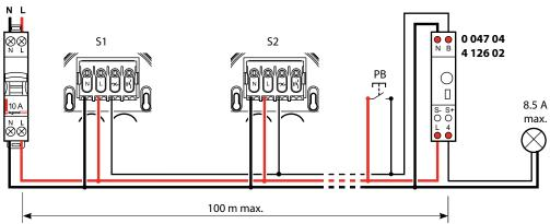
With this wiring, the configuration tool must be on "Pulse" (see paragraph 8. Settings).
