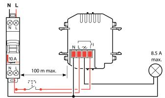
■ 4.2 Wiring without auxiliary control: Auto on/Auto off
