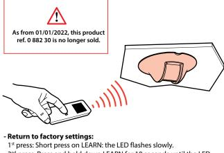
2<sup>nd</sup> press: Press and hold down LEARN for 10 seconds until the LED flashes quickly.
