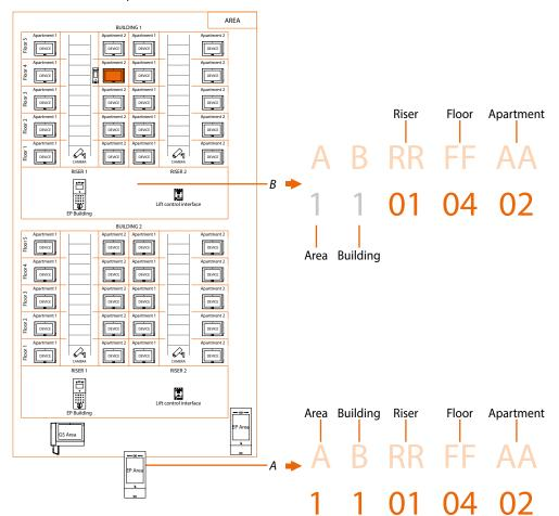
**Note**: during the configuration phase, the number of digits to be used for each call sector (Area/Building/Riser/Floor/Apartment) must be set.
