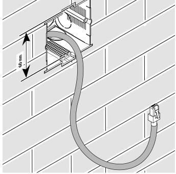
**Attention**: The wrong wiring of the Ethernet cable connecting the device to the Poe Switch 375002 could damage the device itself. The RJ45 cable must be at least 200 mm long.
