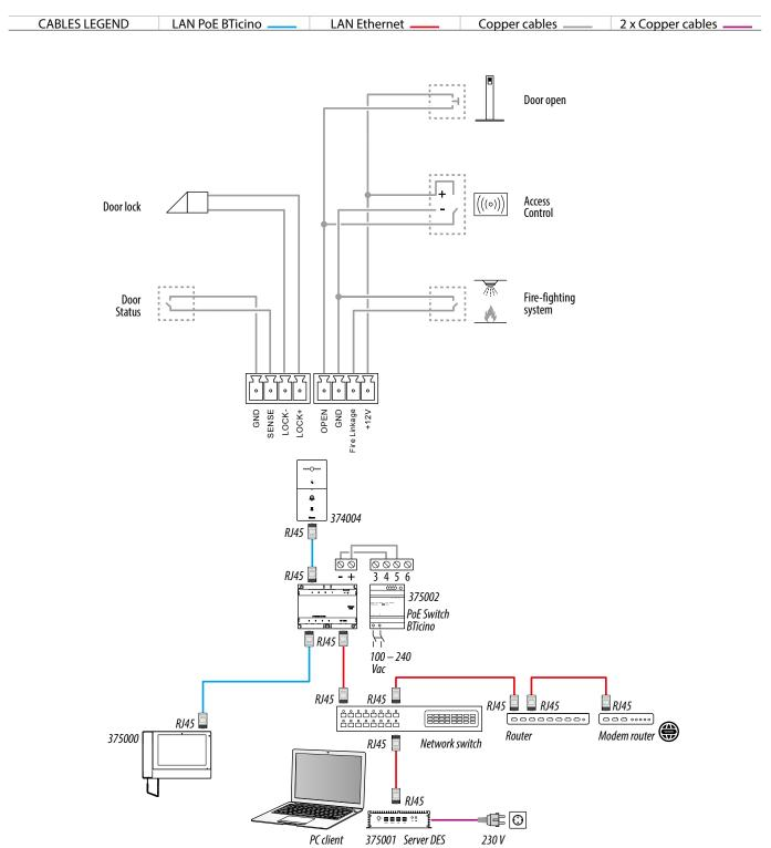
Attention: do not directly connect PoE ports to an unsuitable network interface, such as a device powered by a different voltage. Connect the UP LINK port to a suitable port, never to a PoE port.
