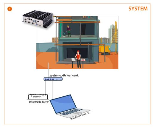
1. Connect the SD to the system LAN network
