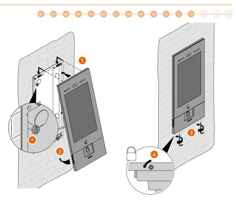
Adjust the tamper screw so that it presses the tamper switch of the device and activates the anti-theft function in case of removal sending an alarm to the guard station.
