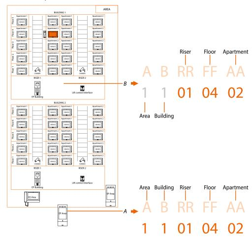
**Note**: during the configuration phase, the number of digits to be used for each call sector (Area/Building/Riser/Floor/Apartment) must be set.
