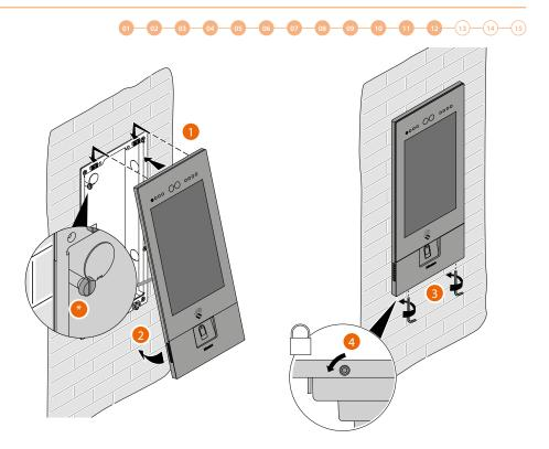
Adjust the tamper screw so that it presses the tamper switch of the device and activates the anti-theft function in case of removal sending an alarm to the guard station.
