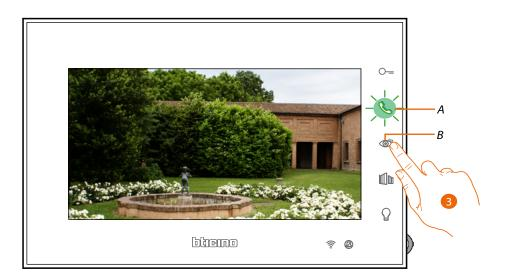
3. Touch to display another Entrance Panel or camera (using the scrolling service). When switching from one camera to the next the key (B) lights up.
