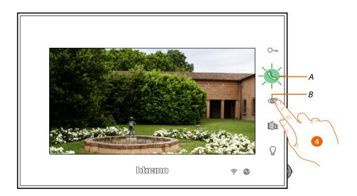
4. Touch to display another Entrance Panel or camera (using the scrolling service). When switching from one camera to the next the key (B) lights up.
