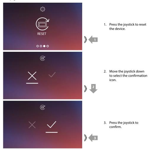
**Note**: all the data concerning associated accounts and the Wi-Fi connection will be deleted. **Note**: this procedure resets the device, to complete the system reset, refer to the Settings/Reset video internal unit section.
