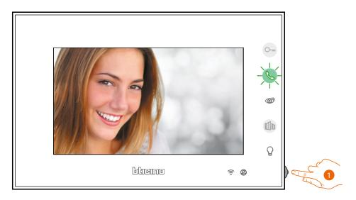
1. If necessary, during the call press the joystick to display the image sound/brightness/contrast/colour adjustment menu (see <u>Audio/video parameter adjustment</u>).
