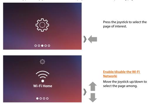
**Note**: to connect the device to the Wi-Fi network and to the app, you must first associate the Connected Indoor Unit to the Door Entry EASY KIT app.
