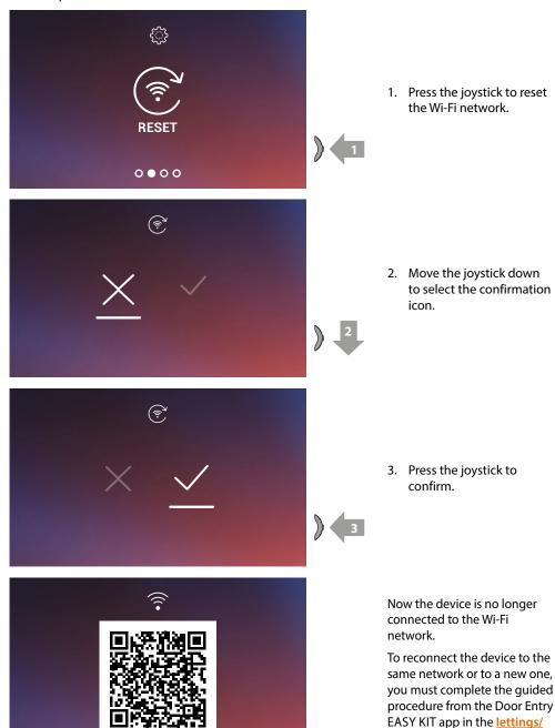
**Note**: if the procedure is not completed, after a few seconds the connection is restored.
