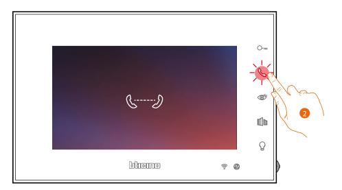
2. When the Internal Unit answers, the key starts to flash; communicate with the Internal Unit, or touch to close the call.
