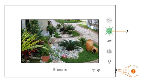
2. If necessary, during the call press the joystick to display the image sound/brightness/contrast/colour adjustment menu (see <a href="Audio/video parameter adjustment">Audio/video parameter adjustment</a>)
