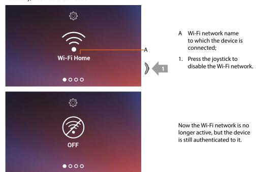
**Note**: to disconnect the Wi-Fi network from the device, the device must be <u>reset</u> following the appropriate procedure.
