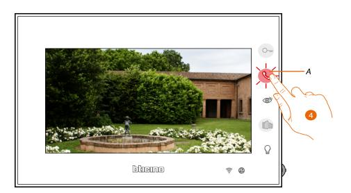
4. The key flashes red, touch to end the communication or wait for the automatic switch off time to elapse.
