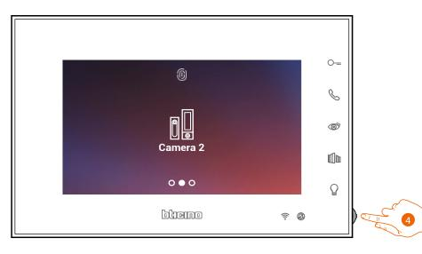
4. Touch to activate the desired camera, (the image is displayed for three minutes).
