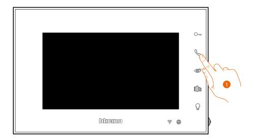
1. Touch to activate the communication with the Internal Unit
