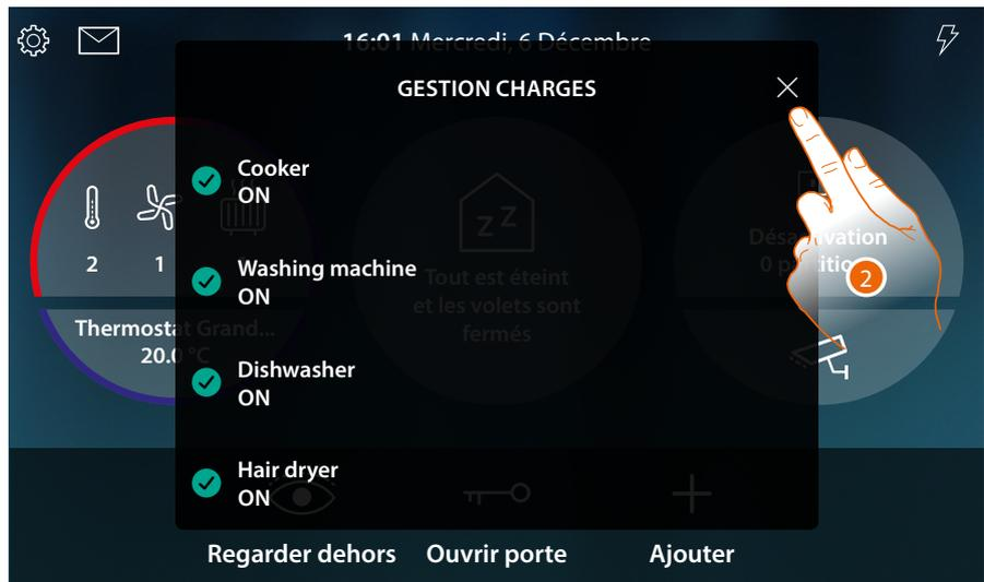
In this page it is possible to view the loads controlled by the control unit and their status:
