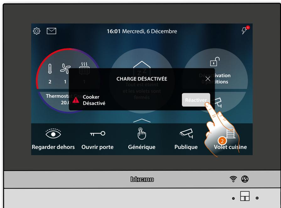
2. Touch to force-enable the load for 4 hours
