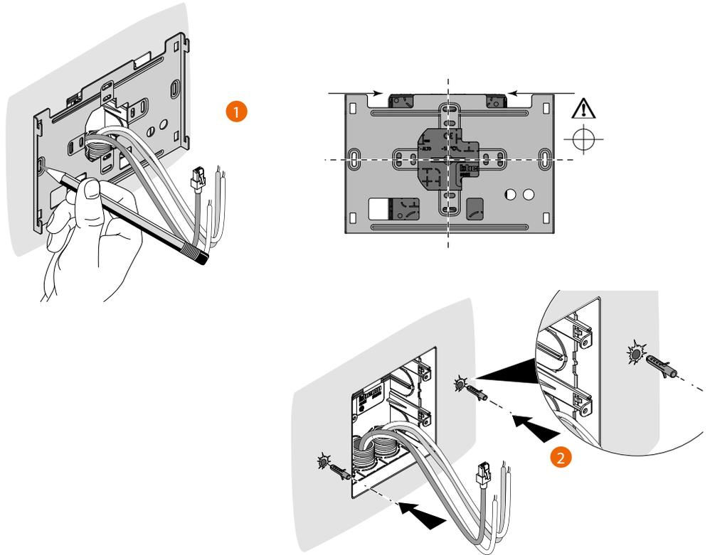
**Caution:** avoid fastening the bracket on uneven or irregular surfaces and excessive screw tightening, in order to prevent any bracket distortion that may compromise the correct installation of the device. The device must slide in the appropriate bracket rails with a slight pressure and without straining.
