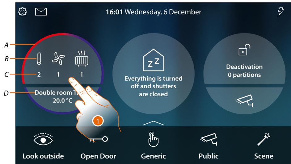
A It indicates through colours (red heating, blue cooling) that at least one of the devices is active
