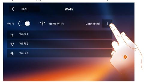
6. Touch to display or modify the network connection parameters.
