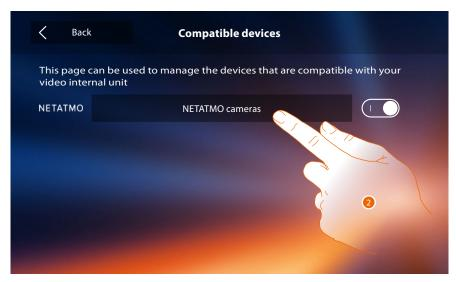
2. Touch to access NETATMO cameras and complete the authentication process.
