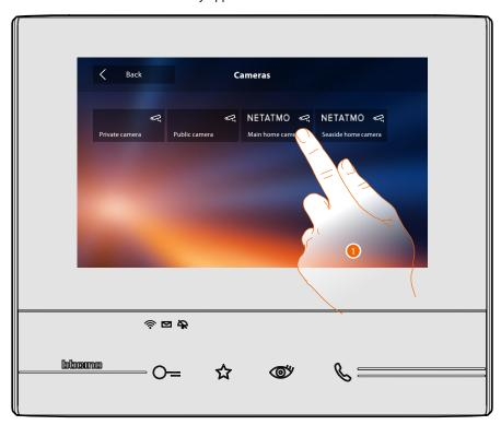
1. Touch to activate the desired camera. (The image is displayed for three minutes).
