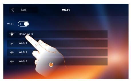
2. Select the domestic network to which you want to connect the device. If the Wi-Fi signal is weak or non-existent check the Wi-Fi installation rules.
