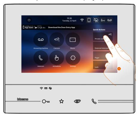
1. Touch to directly enable the function (e.g. camera).
