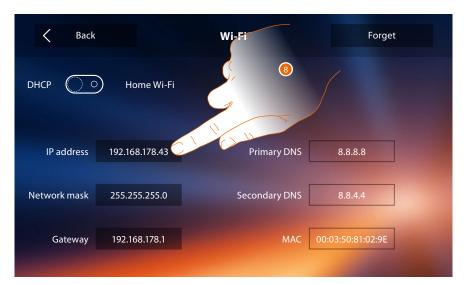
8. Touch to modify the device IP address.
