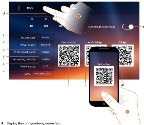
**Note**: the <u>function</u> configurations or modification on the Classe 300X will be automatically reported also in the **DOOR ENTRY APP** after the first association to a smartphone and for any subsequent modification.
