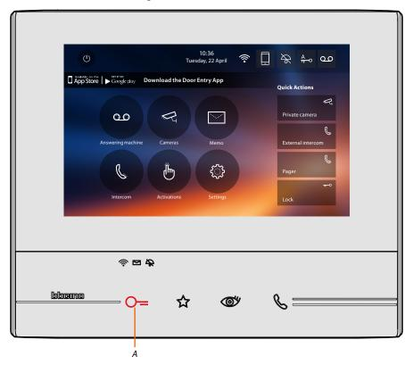
A. LED flashing = door lock open.
