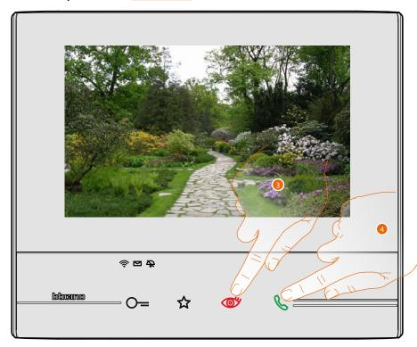
3. Touch to display another camera (scrolling). When switching from one camera to the next, the key lights up.
