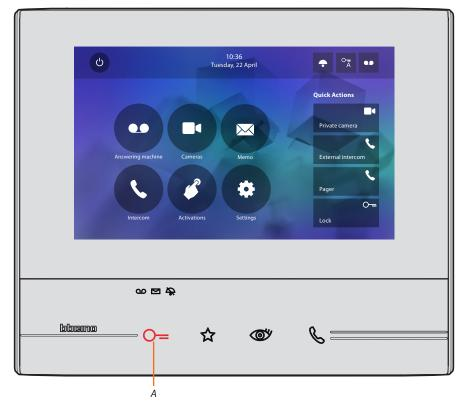
A. LED flashing = door lock open.
