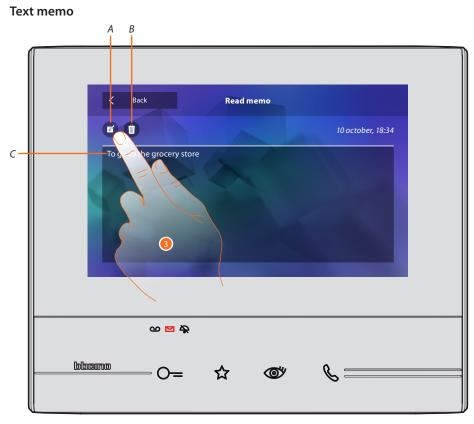
This screen can be used to display (C), modify (A) or delete (B) the memo text.
