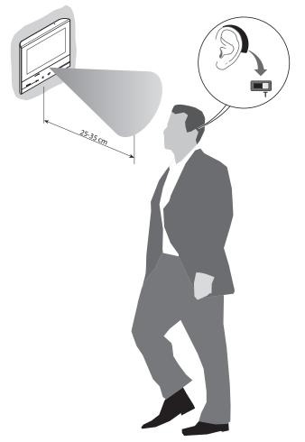
To ensure correct magnetic coupling between the IU and the acoustic device, we recommend a position in front of the device, at a distance of 25-35cm.
