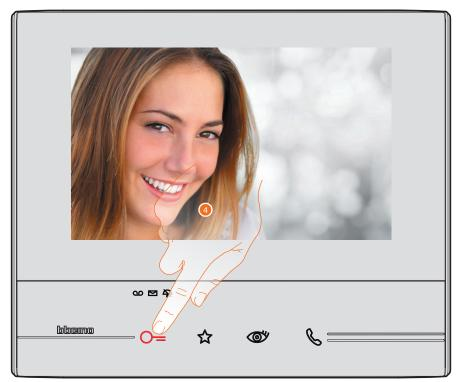
Touch to open the Entrance Panel door lock. The door lock key lights up briefly, to indicate that the door lock has been released.
