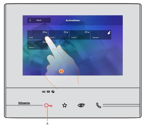
2. Touch to activate the communication with the desired intercom. Key (*A*) lights up to indicate that the activation has been successful.
