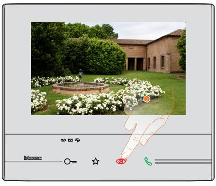
3. Touch to display another camera (scrolling). When switching from one camera to the next, the key lights up.
