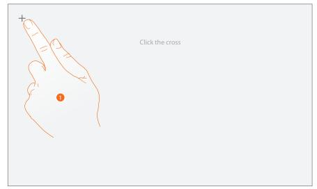
Touch the "cross" symbol on the display as it moves to all 5 positions. At the end, the ok, icons appears at the corners of the display. Touch it to complete the calibration procedure.
