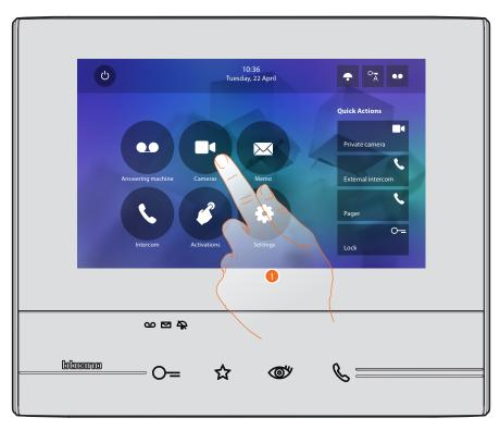
This section can be used to monitor your home by enabling one of the video surveillance system cameras inside the apartment or the common areas (e.g. garages, garden).
