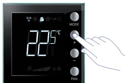
Set the desired temperature using + or -; the display will show the symbol
