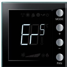
**NOTE:** if ER4 or a temperature very different from the one felt are displayed, or after the first installation, wait at least 5 hours before checking the operation again. If the problem continues, contact a trusted technician.
