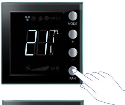
The display brightness can be adjusted on 10 levels. Press the FAN key for at least 7 seconds.
