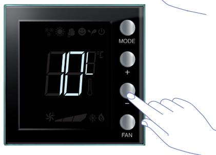
The current brightness level appears on the display. Use the + and - keys to increase or decrease the brightness.
