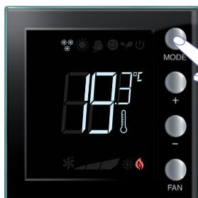
To switch from normal operation to Antifreeze (or thermal protection) press the **MODE** key.
