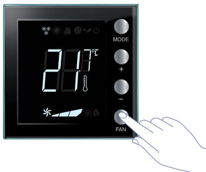
Press **FAN** to set the fan speed at the desired level.
