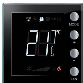
After a few seconds the new set-point is saved and the measured temperature appears. In this example the set temperature is higher than the measured temperature, therefore also the heating on indicator will come on
