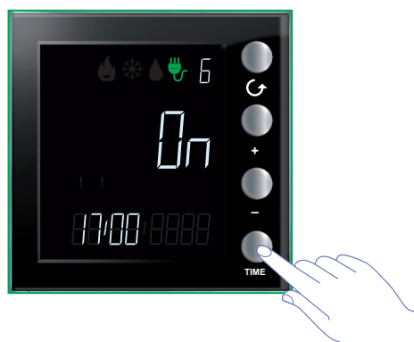
E.g. status of the load on line 6
