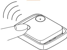
Press one of the radio remote control keys. Whenever the remote control has already been saved the control unit will return to the list of keys showing the existing one in case you want to modify it.
