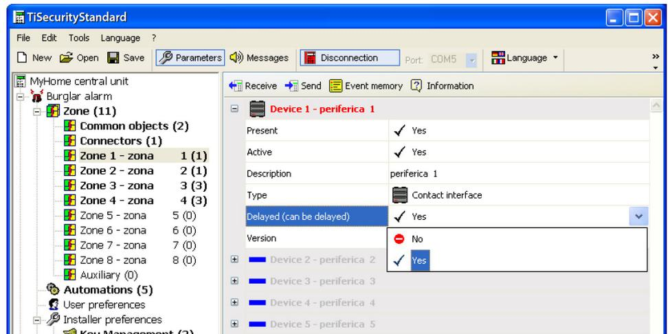
When you click the Information button, you will see a screen which will show how the delay time will be set up for the devices of the zone.
