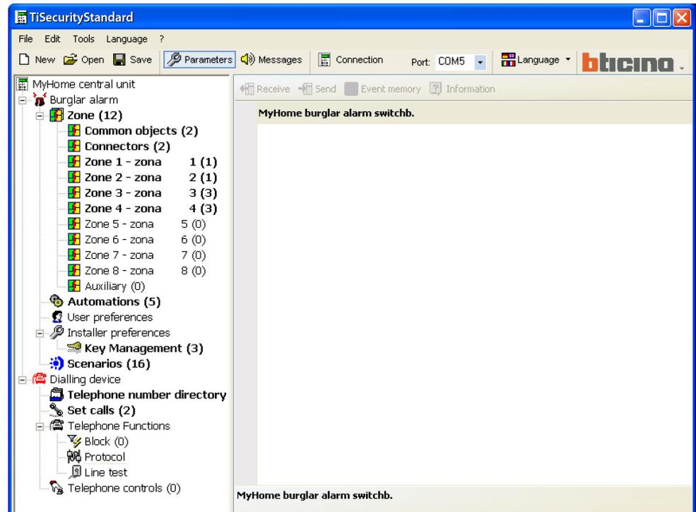
In this section all typical parameters for the configuration of the Unit are displayed, represented hierarchically with a tree structure on the left side. On the right side, a specific template for inputting data and, if the connection is active, for communicating with the Unit can be displayed by selecting each element of the hierarchic structure.
