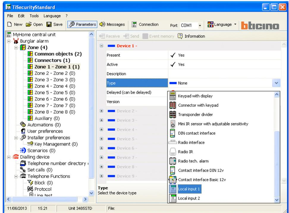
After assigning the contact to the zone, the contact mode can be set.
