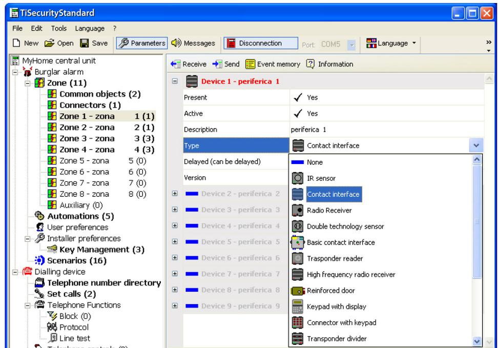
Furthermore, it is possible to enable/disable the activation delay the device can be delayed or not depending on the type of device selected and on its firmware version.
