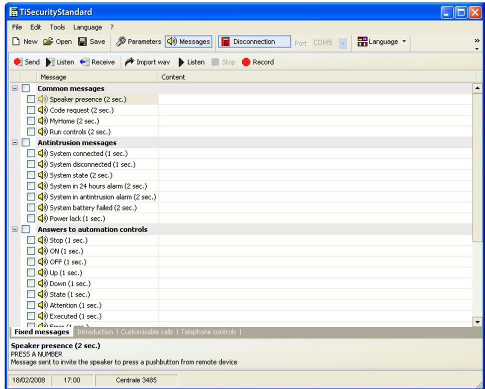
The screens in the “Messages” section display the messages related to the type selected in the bottom menu (fixed Messages, Presentation, customizable Calls, telephone Commands); it is possible to select the various templates by clicking the corresponding buttons.
