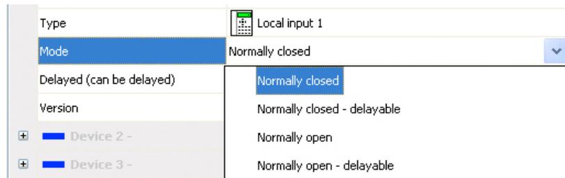
For the operating modes with “delay” function, the activation delay time will be the same as the one set in the User Preferences menu.
