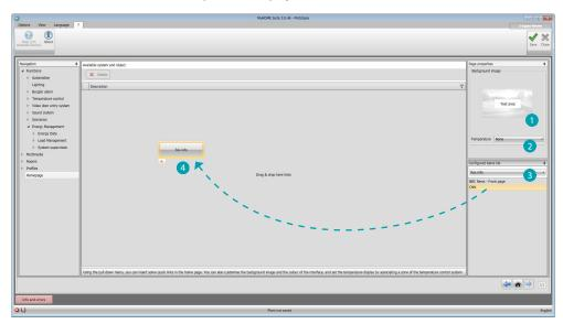
Select the image that you want to appear on the Home Page of the device 1 and the zone from which to detect the temperature displayed 2.
