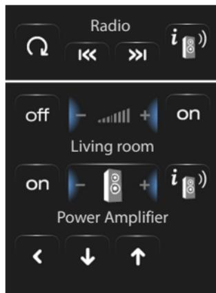
ON/OFF icon, to switch the power amplifier on or off
