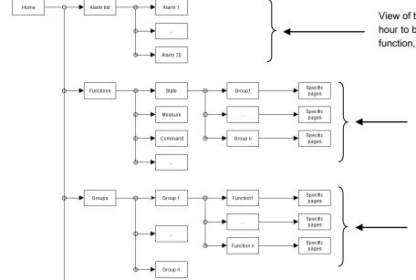
View of the 20 last alarms: status fault, date and hour to be set up , measure threshold, duplicated function, communication fault,...
