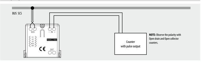
WARNING: The pulse counter interface must be installed as close as possible to the power supply unit, to ensure a high BUS voltage and enable correct management of memory savings in case of power failure. If the supply voltage is insufficient (below 21 Vdc), the pulse counter interface will
