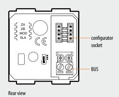
**NOTE:** compared with the previous version, the P and DEL configurator sockets have been removed.
