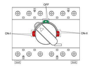
While switching OFF, if handle does not rotate & stays in ON position or between ON & OFF position at source-I (ON-1) as shown above, then it indicates welding fault.
