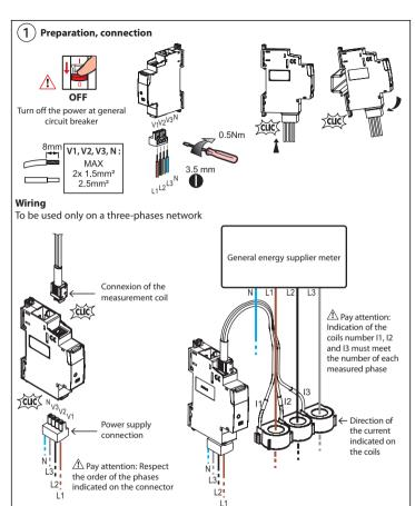
The module is powered from 100 to 240V~ between Neutral (N) and Phase 3 (V3).
