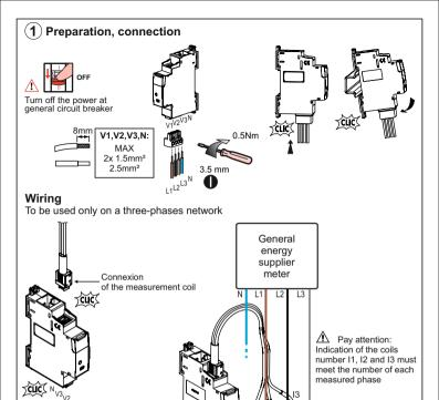
The module is powered from 100 to 240V~ between Neutral (N) and Phase 3 (V3)
