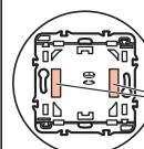
Stick the 2 repositionable adhesives on the back of the wireless control
