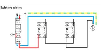
Replacement of an existing 2-way switch by a connected switch + wireless light switch
